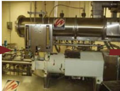
An example of an Extruder needed to make puff product
